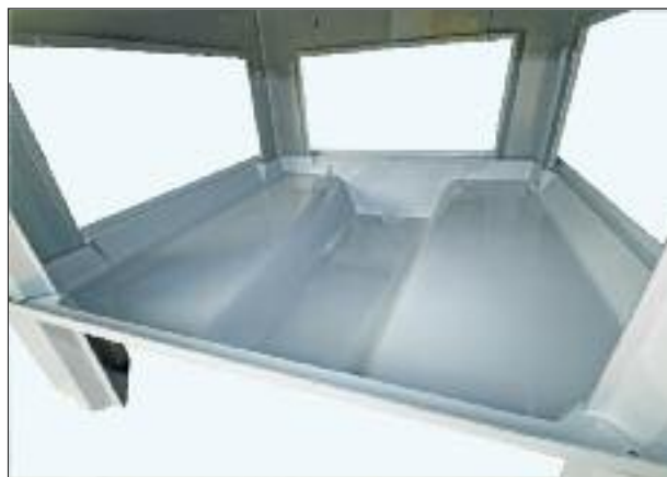
Compound curvature provides innate part strength
